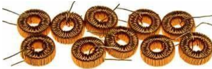
Inductors on a toroidal ferrite former
